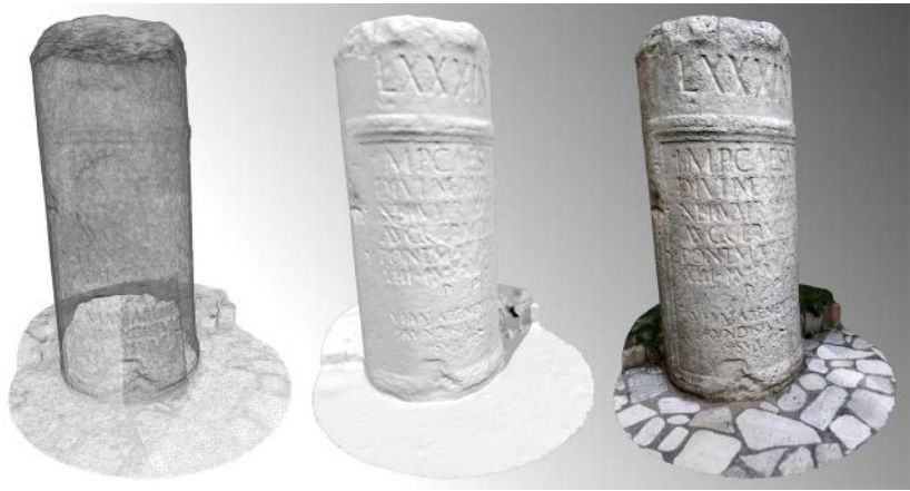
Fig. 26.6. The 3D model of the Roman milestone elaborated with Autodesk 123D Catch (wireframe – smooth – texture rendering)
