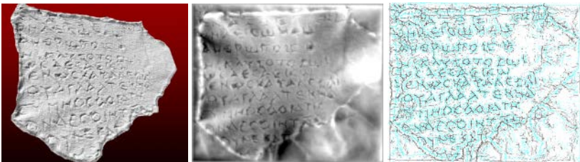
Fig. 27.2. The Digital Epigraphy Toolbox offers different visualizations of the same 3D digitized inscription. Left: 3D visualization, Center: depth-map (deeper inscribed areas appear darker), Right: fingerprint-map (visualizes local peaks and valleys in cyan and black respectively).
