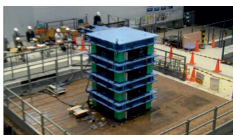
Figure 1: Shake table test experiment for wireless sensor performance.
