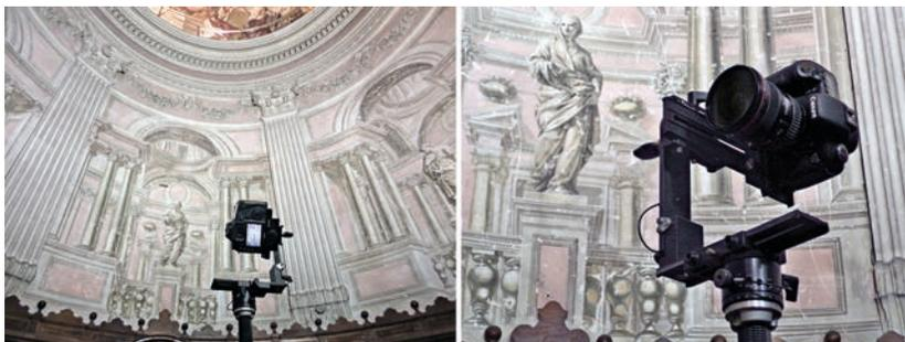
Fig. 5. Panoramic head and camera used for photographic capture.
