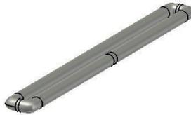
Fig. 3.6. Numerical model of a cylindrical folded dipole. One of the two arms is suitably cut to allow for the introduction of an idealized voltage gap.
