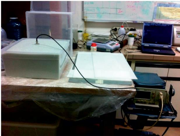
**Fig. 5.4.** TDR measurement setup to control the conductivity variation due to change on the KCl concentration. Copyright © 2017, IEEE.
