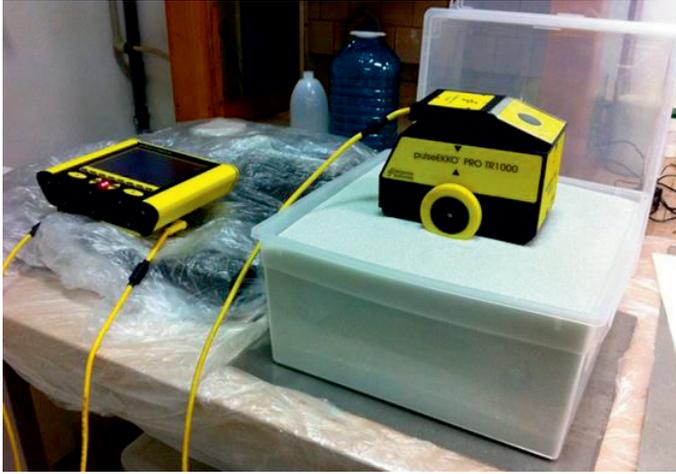
**Fig. 5.3.** An experimental laboratory setup for the analysis of ETS features, developed at the applied geophysical lab of 'Roma Tre' University. An air/dielectric environment is investigated by means of a simple commercial GPR system with interfacial fixed close antennas. The ground dielectric constant and conductivity can be changed in controllable ways. Copyright © 2016, IEEE.
