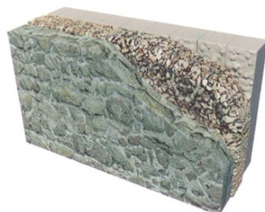
Two faces wall (one on stonework masonry and another on ashlar stone masonry) with internal filler
