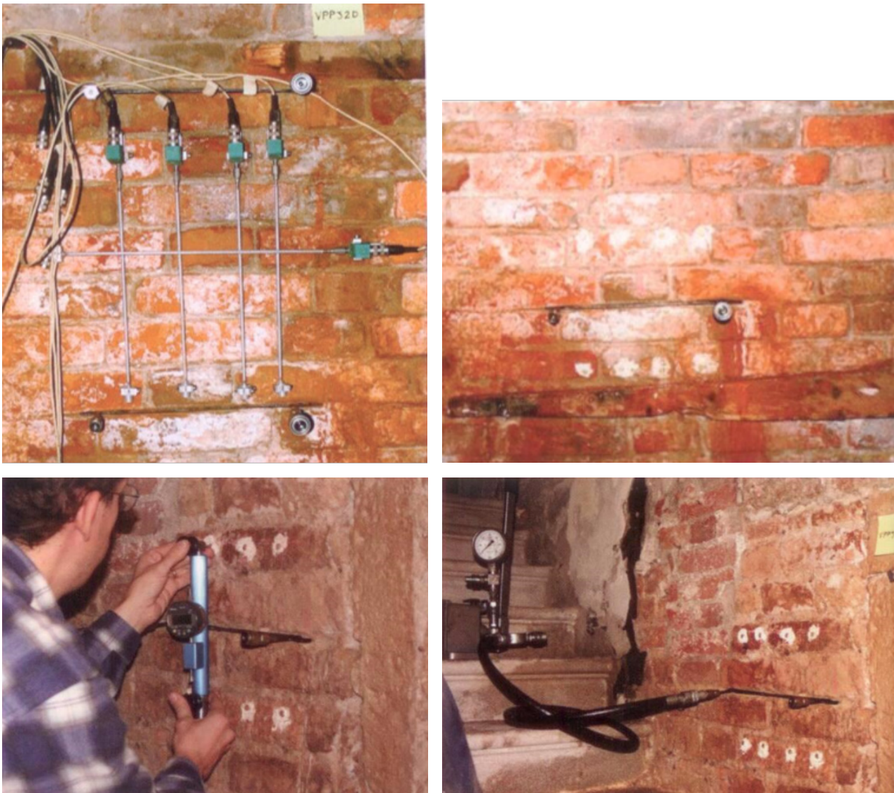
Fig. 5. Reading of the vertical movements with the flat jack inserted in the masonry wall. Hydraulic system connected to the flat jack inserted in the masonry wall. From F. Doglioni, G. Mirabella Roberti, Venezia. Forme della costruzione, forme del dissesto , Libreria Cluva Editrice, Venezia 2011, p. 208.
