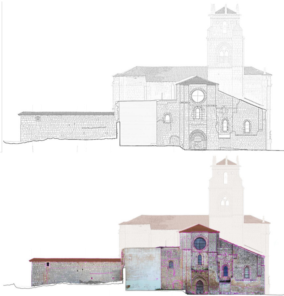
Fig. 28. Material survey and Phase-delimitating lines of Santa María la Real Church, Sasamón, 2014. (6)
