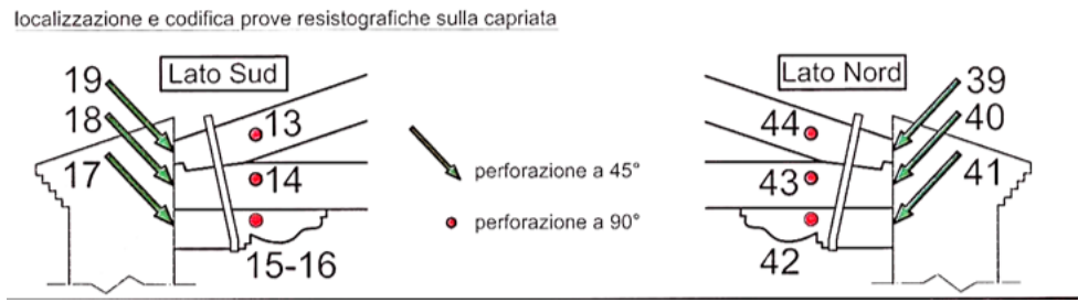
Fig. 56. Analytical diagnosis data card including: list of damages, location and codification of test performed on the truss and typological recognition of wood species. Redesigned by Susana Mora.
