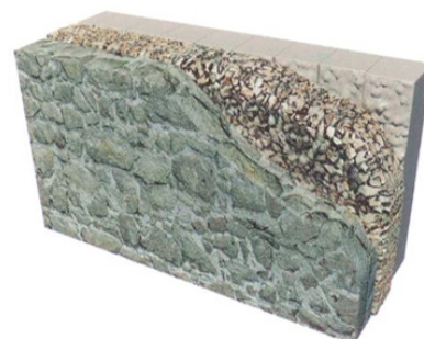
Two faces wall (one on stonework masonry and another on ashlar stone masonry) with internal filler
