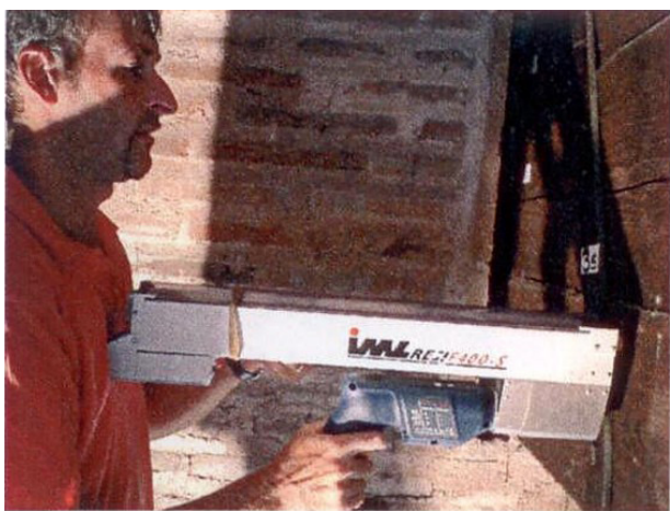
Fig. 62b. Perforations with resistograph in span (left) and in correspondence of the support (right). From P. Rocchi, C. Piccirilli, Manuale della Diagnostica , Edizioni Kappa, Roma 1999.
