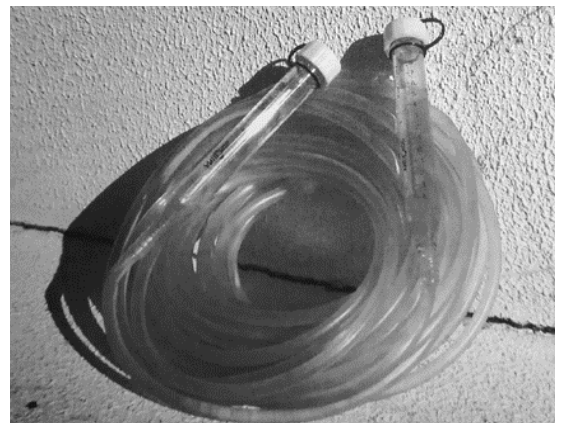
Fig. 4. On the left: paper, pencil and measuring tape. On the right: water level. Photos by Susana Mora.
