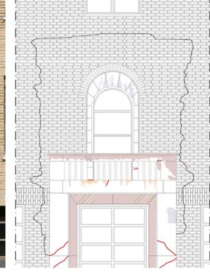
Figure 15/16 - Identification of the area of Litoceramic cladding characterized by mortar of different colours; graphic representation (© Santarelli, Giorgi, Ciacchella, Pandolfi 2020)
