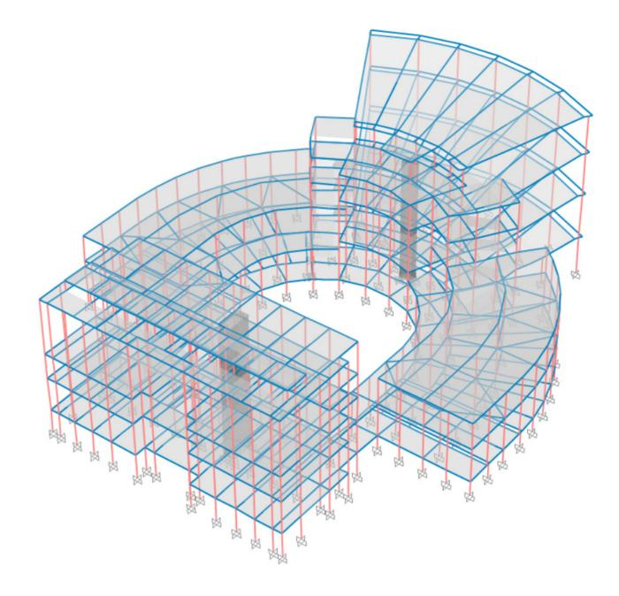
Figure 40 - 3D model of the building in its original configuration in 1935 (© Martella 2020)
