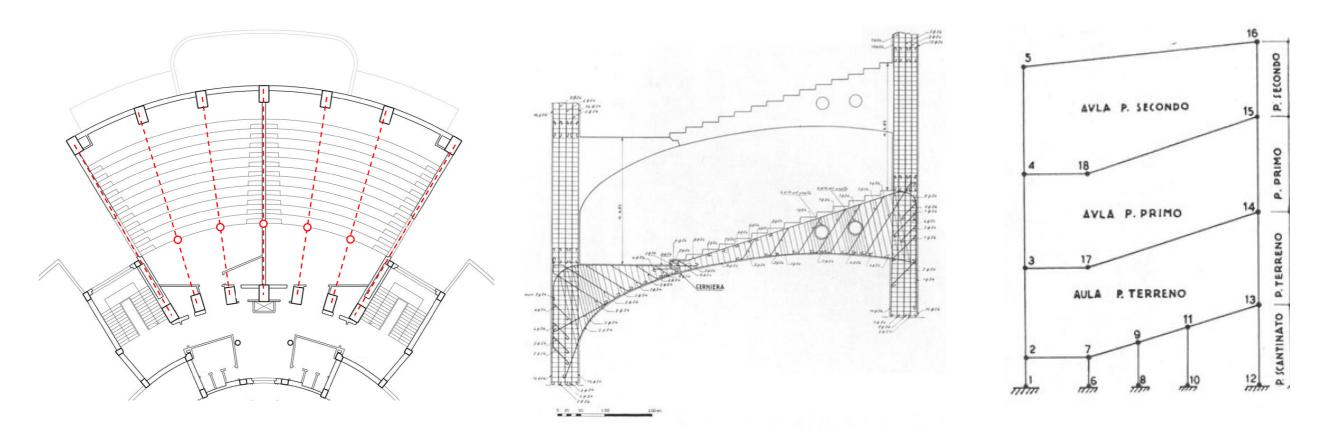
Figure 19 - Schematic representation of the beams at the intermediate levels of the tower of classrooms
