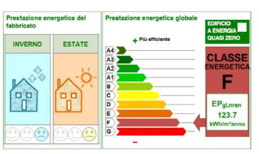
Figure 35 a/c - Energy Performance Certification of the front building, curved wings and tower of classrooms in the current condition (© Mancini, Romano, Rosso 2020)
