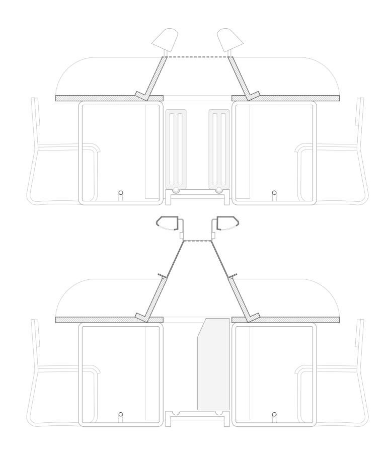
Figure 18 a/b - Reconstruction of the original situation and current condition with modifications due to the change of the lighting fixtures and the embedded radiators with fan coils (© Cortesi 2021)
