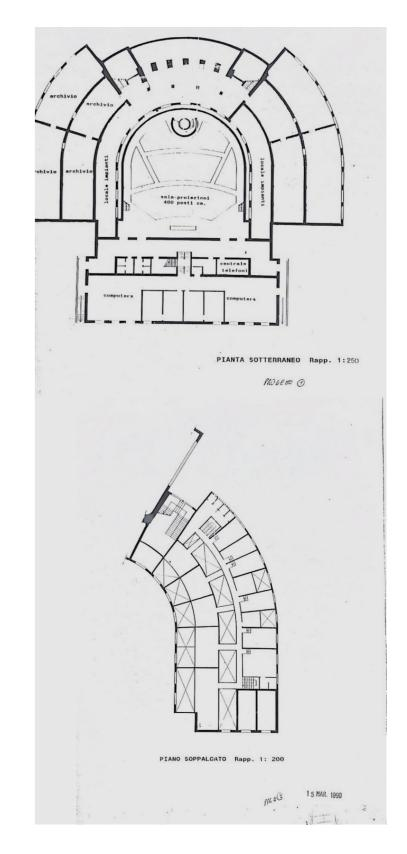
Figure 8 - Project for an assembly room created by excavating the inner courtyard of the School of Mathematics, 1990 (ADM\_drw\_04)
