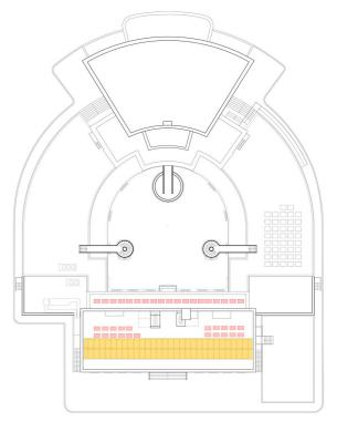
Waterproofing of the library roofing with restoration of the skylight, reorganization of the interiors and requalification works of the professors' sitting room and installation of the photovoltaic equipment (additions in red and removals in yellow)
