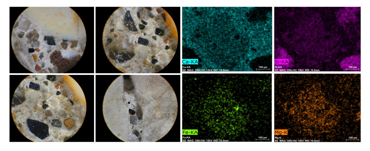
Figure 5 a/d - 7x microscopic observation of a concrete resin-embedded sample collected on the crowning frame (© Santarelli, Giorgi, Ciacchella, Pandolfi 2020)
