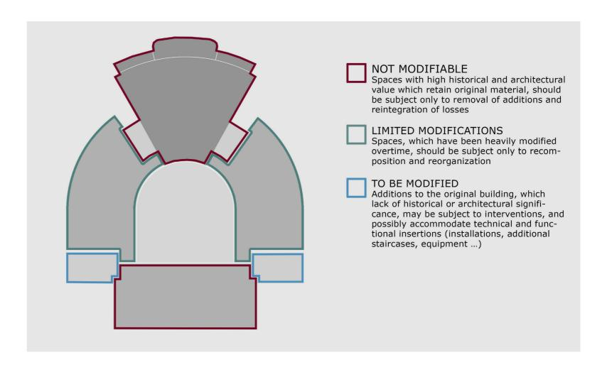
Figure 9 - The three blocks of the building have been modified over the years, albeit each in a different manner (© Salvo 2021)
