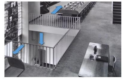
Figure 14 - Detail of air flow in the library reading hall in the original situation (ACS\_pht\_30)
