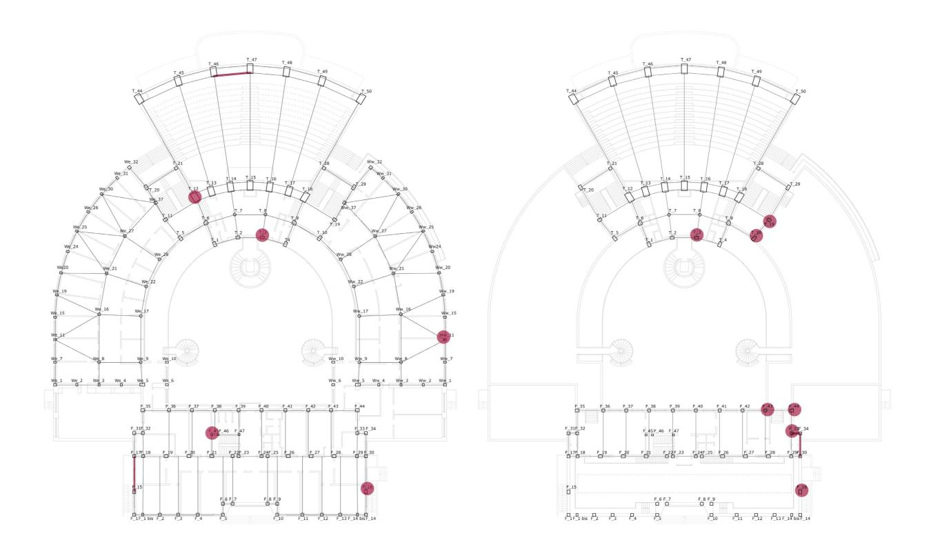
Figure 47 - Not satisfactory structural elements: first level (© Martella 2020)
