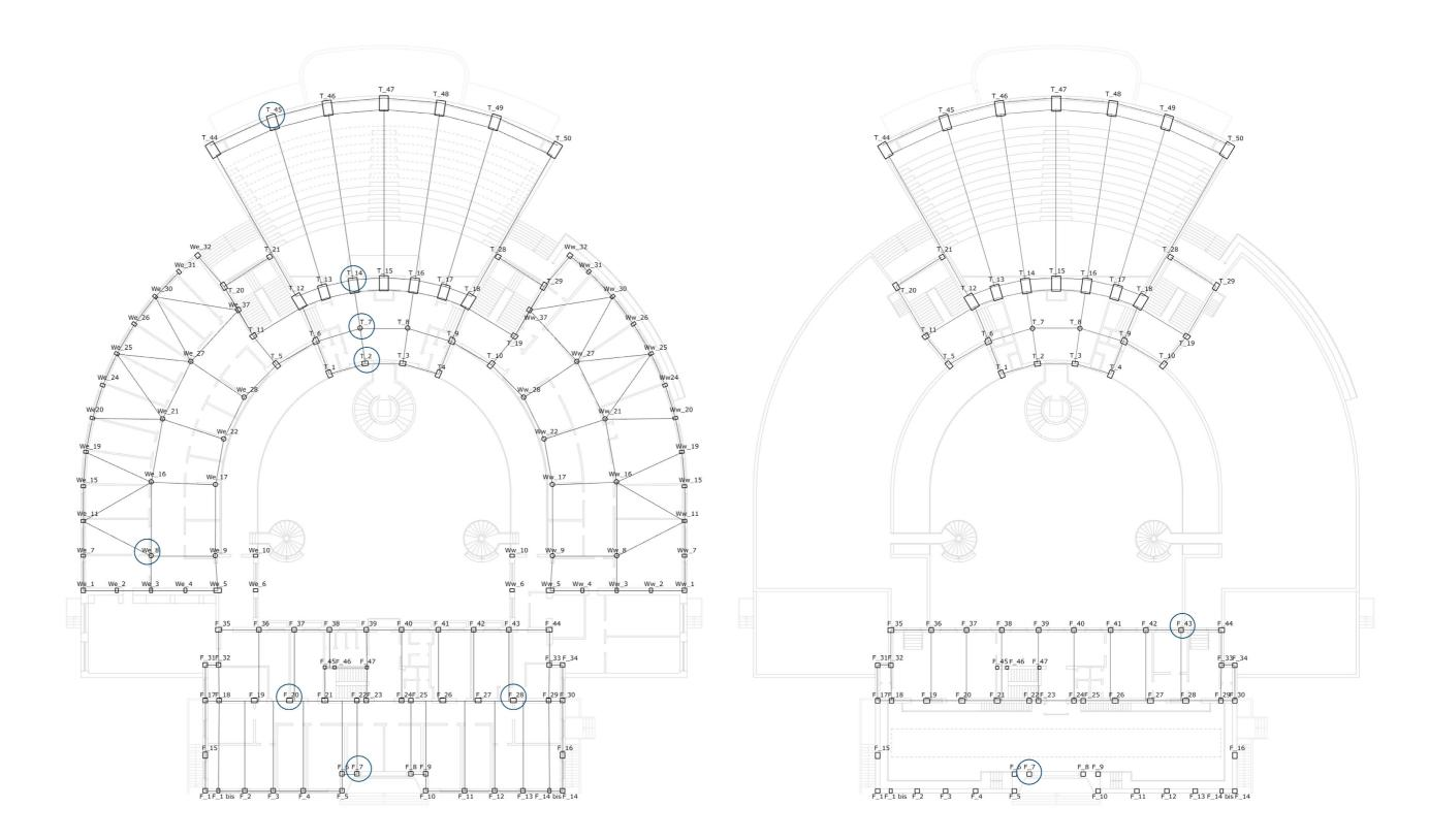
Figure 9 - Structural elements identification numbers and location of the rebar locating tests, first level (© Martella 2020)
