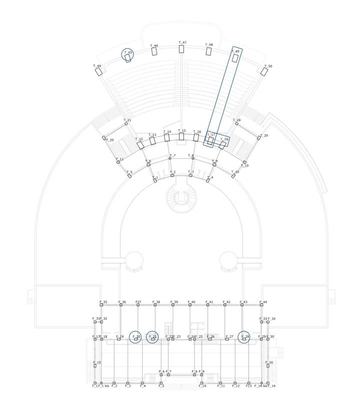
Figure 11 - Structural elements identification numbers and location of the rebar locating tests, third level (© Martella 2020)
