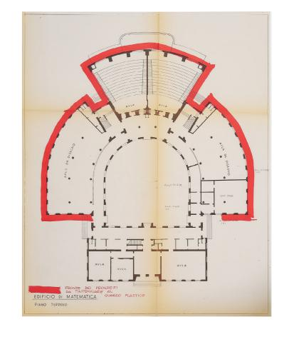
Figure 5 - The ground floor of the School of Mathematics; the bold red line indicates the surfaces to be repainted "with plastic quartz", 1980 (ASS drw 162).
