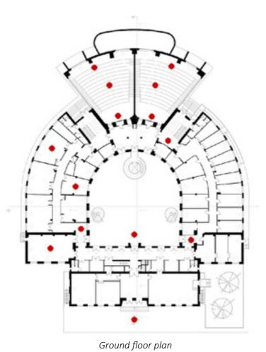
Figure 34 - Positioning of measuring points for IAQ sampling at the three levels of the building (© Mancini, Romano 2020)
