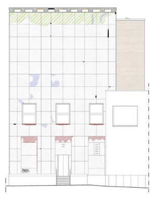
Figure 9 a/b - Analysis and mapping of the state of conservation of the travertine slabs cladding; north, east and west elevations (© Santarelli, Giorgi, Ciacchella, Pandolfi 2020)
