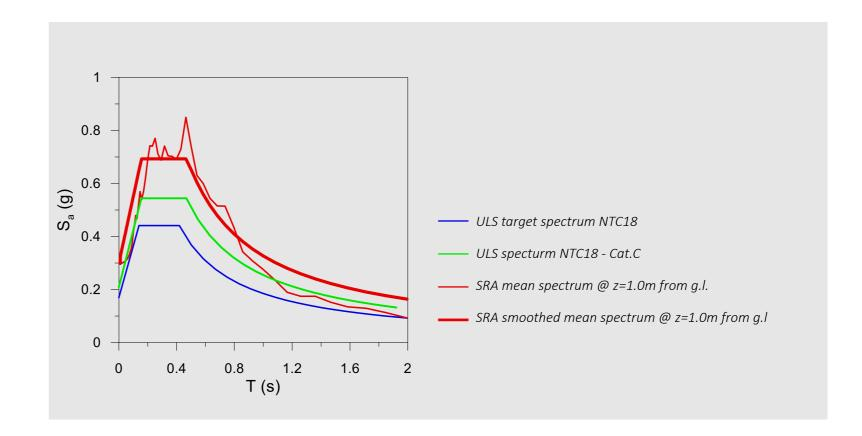
Figure 9 - Average response spectrum and average smoothed NTC18-type response spectra calculated from 1D site response analyses along with target and subsoil category C spectra from NTC18 (© Lanzo 2021)
