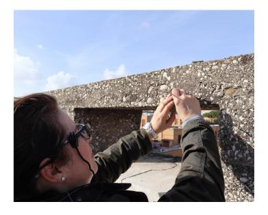
Figure 16 a/b - Collection of microscopic samples for laboratory analyses performed by Task Group 3 (© Pandolfi 2021)
