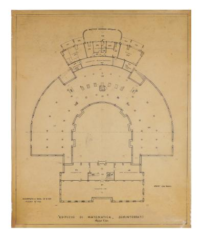
Figure 1 - Plan of the basement designed by Ponti in June 1935; details are provided regarding the house of the porter and his family, located at the foot of the classroom tower with its systems and garages (ASS drw 69)
