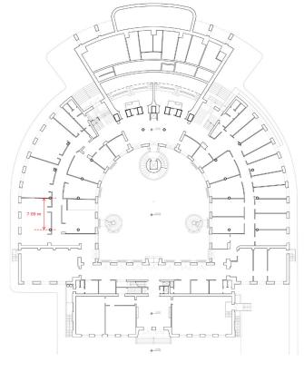
Figure 10 - Plan of the ground level as of December 18, 1933 (ASS\_drw\_25). Columns highlighted with red circles are not present in a drawing dated 1935 as well as in the building
