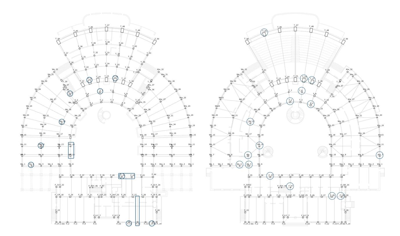
Figure 7 - Structural elements identification numbers and location of the rebar locating tests, basement level (© Martella 2020)
