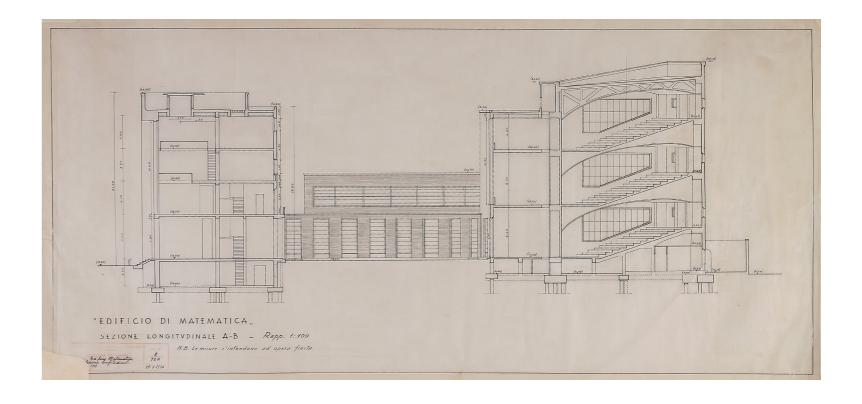
Figure 4 - Longitudinal section of the front building, drafted by Ponti in January 1934; it is easy to see that he envisaged a direct link between the corridor, the professors' lounge and the library (ASS\_drw\_33)
