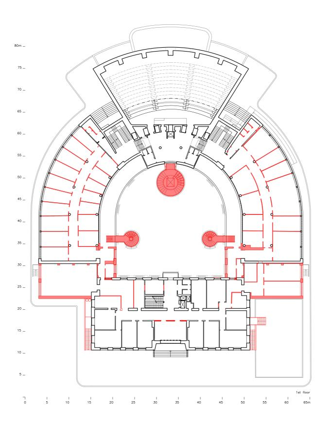
Figure 4 - Additions to the building from 1939 to 2021; plan of the first floor (© Cortesi 2020)
