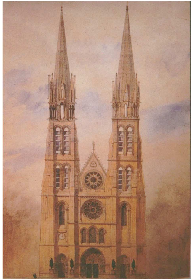
Fig. 14. Paris, Saint-Denis abbey, drawing for unity of style by Viollet-le-Duc. The façade in a restoration project drawing made in pen and watercolour, 1870, signed by Viollet. (In Ibidem , p. 42)
