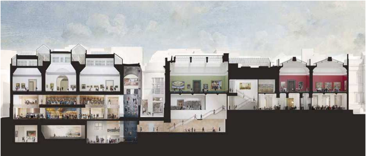
Fig. 24 - Cross-section perspective looking north through (from the left) the Sainsbury Wing and Wilkins rooms. (By Selldorf Architects page)
